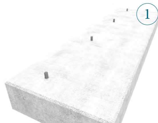
1. Drill, vacuum, insert glue and chemical anchor.
